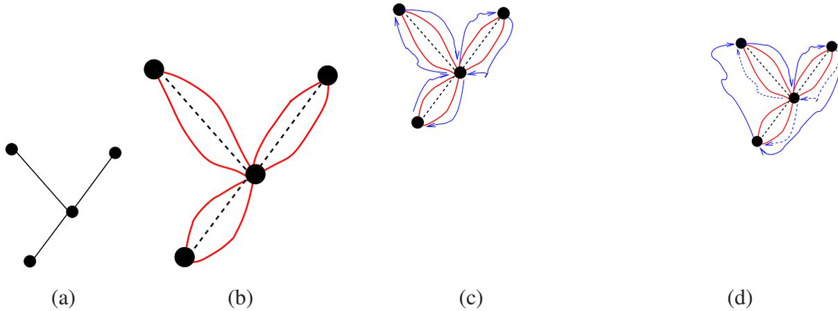
Figure 7.3: The TSP approximation algorithm: (a) the input, (b) the duplicated graph, (c) the extracted Eulerian tour, and (d) the resulting shortcut path.
