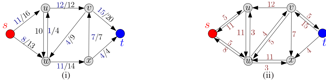
Figure 15.2: (i) A flow network, and (ii) the resulting residual network. Note, that f(u, w) = -f(w, u) = -1 and as such c_f(u, w) = 10 - (-1) = 11 .
